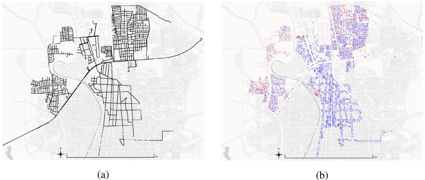
Fig. 18. Screening at Juchitán de Zaragoza, Mexico: (a) Data collection routes (b) Screened building: blue is confined masonry buildings and red is unconfined masonry buildings. (For interpretation of the references to color in this figure legend, the reader is referred to the web version of this article.)
